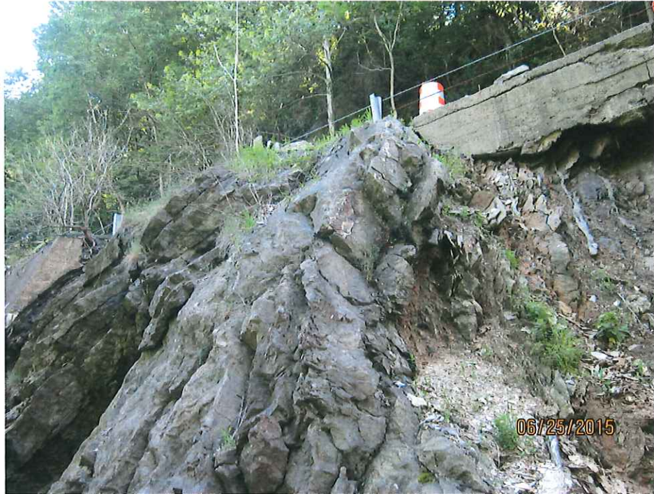
2-5. Close-up of outcrop of competent bedrock on east side of fracture zone.
