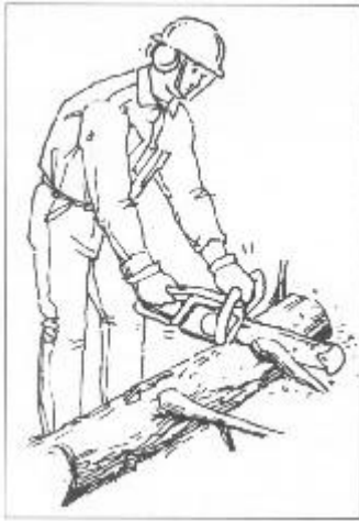
Figure 6: Cutting limbs on top first
